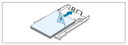
• Load a stack of envelopes with the flap up and to the right.
